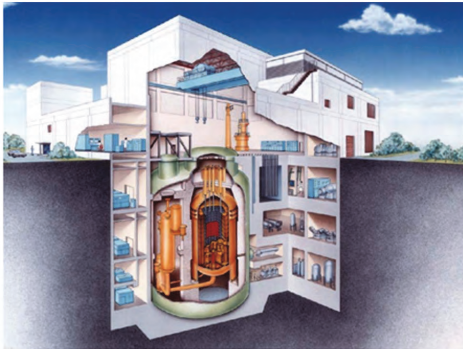
Fig.1 (Japan) HTTR Cross Section
